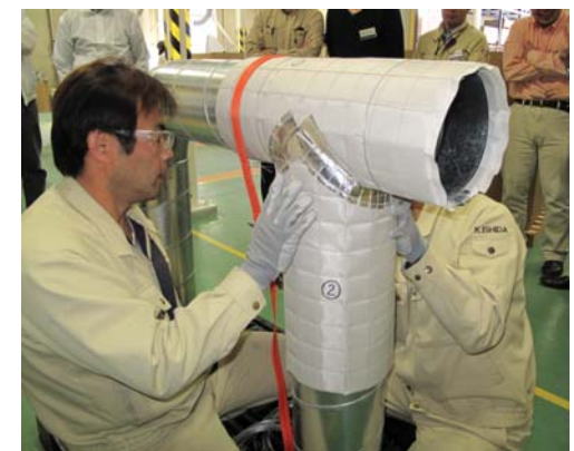
Left: A recent demonstration of MICROTHERM® Overstitched on cross over pipes in their Nagoya factory
