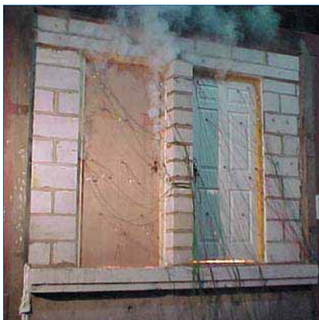
ABOVE: An AS1530/4 type standard fire resistance test incorporating two proprietary fire doors under fire test.
