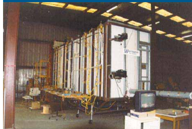
ABOVE: Warrington Fire Research test methodology FSE021 that is used for combined and dynamic fire and smoke leakage measurement. It incorporates a standard fire resistance test furnace and an adjacent full-scale corridor arrangement.
