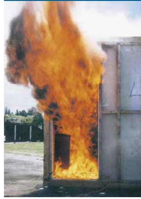
Fire starting in the compartment furnished as a lounge (above). Flash-over occurring less than 3 minutes after the fire started (below), when the heat is so intense that everything in the room ignites and the fire explodes out of the room openings.
