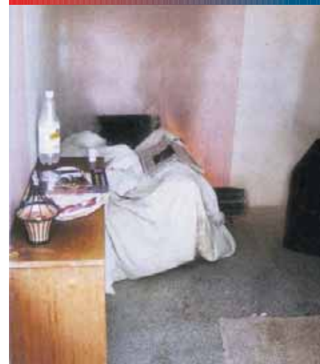
Fire starting in the compartment furnished as a lounge (above). Flash-over occurring less than 3 minutes after the fire started (below), when the heat is so intense that everything in the room ignites and the fire explodes out of the room openings.
