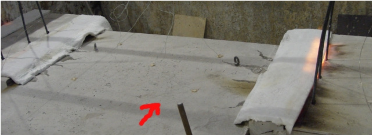
The specimen after eight minutes of heating. Notice the radial crack pattern on both sides of the specimen (with moisture emerging). With some difficulty, the dry crack adjacent to the middle wall can already be seen here, where the arrow points.
