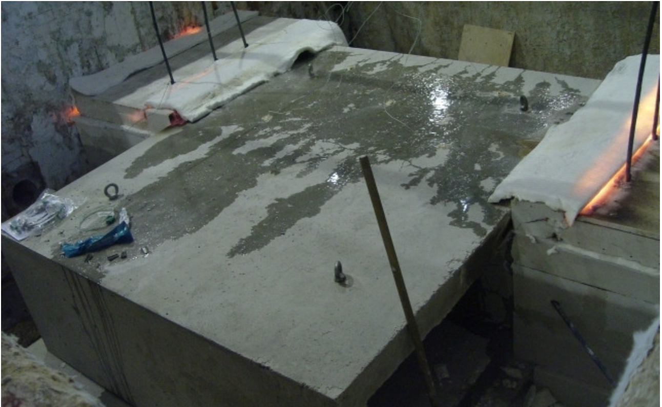
The specimen after 20 minutes of heating. The amount of water emerging from the cracks has become so large that it is now flowing toward the unheated side, even though no cracks appear here.
