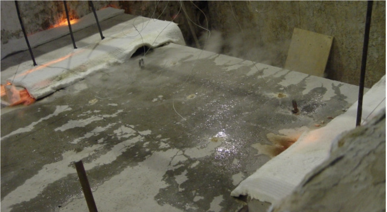
The specimen after 30 minutes of heating, when the water on top of the specimen is boiling. Notice how clearly the crack adjacent to the middle wall stands out now.
