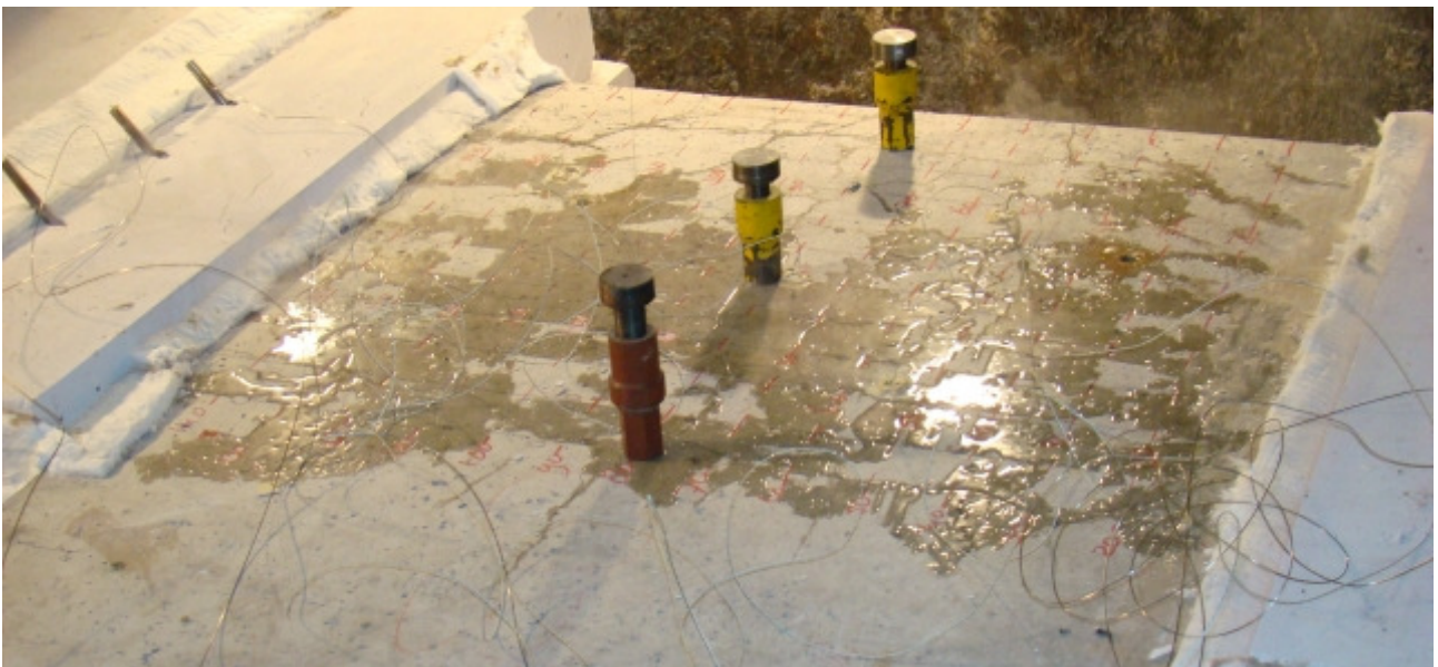
The specimen with fibres 18 \mu\text{m} in diameter and 12 mm in length after 30 minutes of heating. Note the relative scarcity of water compared to the test without fibres.
