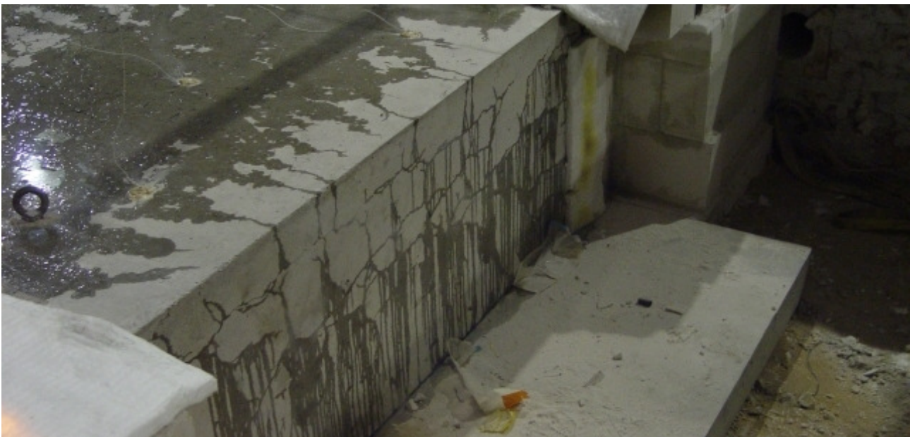
A photograph from the reverse angle showing the side wall of the picture after 20 minutes of heating.
